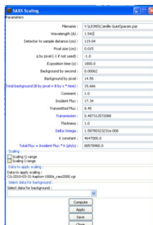
Figure 4.4: Example of SAXS scaling parameter file from PySAXS software
